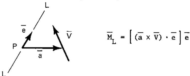
In the figure above,  $\bar{e}$  is a unit vector along line L-L, P is a point on the line, and  $\bar{a}$  is an arm from P to the vector  $\bar{V}$ .
