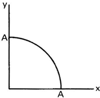
Find the first moment of a quarter of a circular arc of radius  $a$  about the  $x$ -axis.
