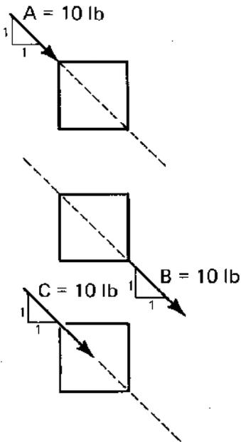
For example, force A has the same external effect on the body as force B or force C, since all three forces have the same line of action. Thus we could say that A, B, and C are "equivalent" forces.
