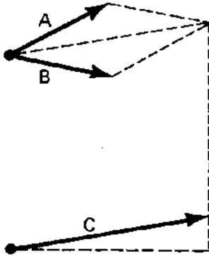
This means that forces A and B acting together on a particle have exactly the same effect on the particle as force C which is proportional to the diagonal of the parallelogram constructed on forces A and B. Force C is called the resultant of A and B. This is an observed law. It cannot be proven mathematically.
