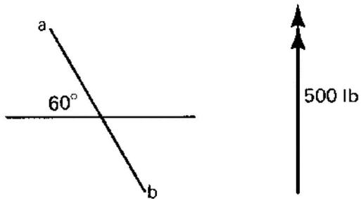
Break the 500 lb force shown into two components, one horizontal and one parallel to ab. Solve the problem trigonometrically and check your answer graphically.
