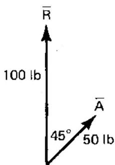
$\vec{A}$  is one component of  $\vec{R}$ . Find the component which, when added to  $\vec{A}$ , will produce  $\vec{R}$  by a trigonometric solution. Then check it by drawing the figure to scale and measuring.
