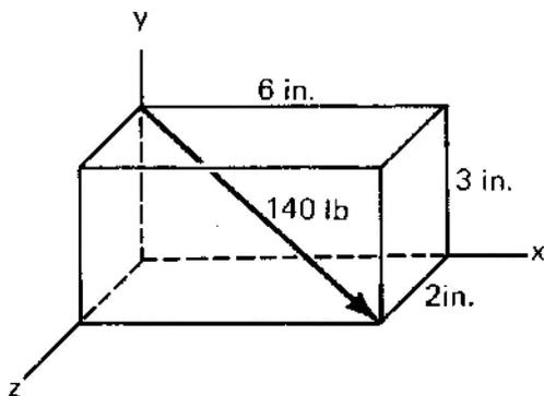
Break the force shown into three components, each of which is parallel to a coordinate axis.
